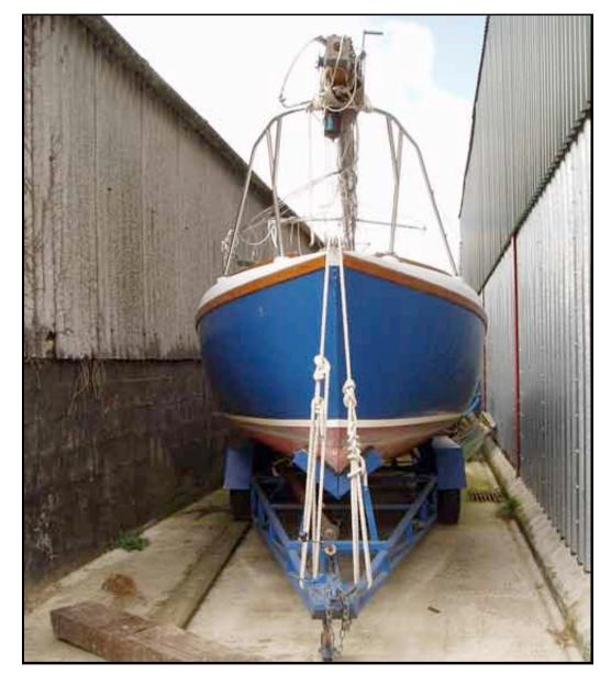
Helene is a Fairey Atalanta designed by Uffa Fox and built by Fairey Marine in 1960. Construction of hull and superstructure is hot moulded Agba. Windows are Perspex.
