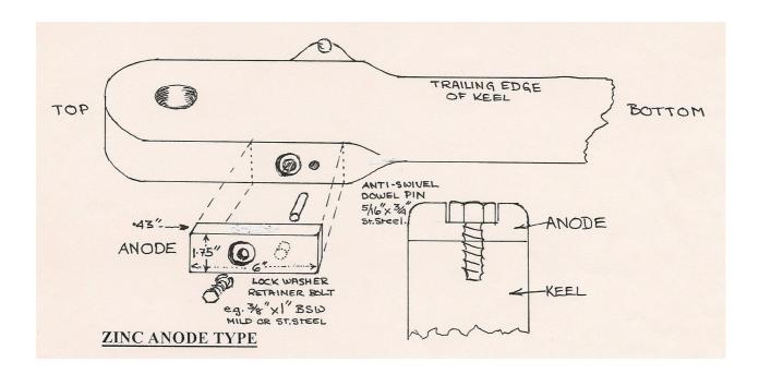
Note – Anodes can be fitted with the keels in the boat.
