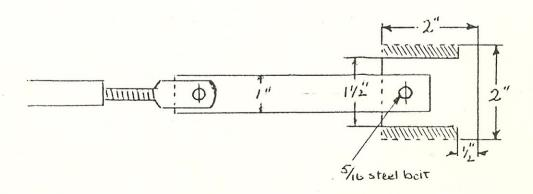
The schematic diagram shows an extractor which was used in the same way as described in Section 4.2(d).
