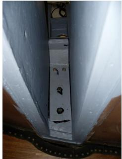
Then offer up the two pressure plates and get an assistant to pass the upper and forward keel bolts through the circular cut-outs forward of the main bulkhead, and fit the nuts loosely onto these bolts. I coat both sides of the pressure plates liberally with grease before fitting them, but be careful not to drop them – you will have your head in the way if they slip out of your
