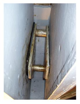
hands. Now press each plate outwards so that the gap for the keel to fit into is as big as it can be. The last bolt which the keel pivots on has to be left out at this stage.
