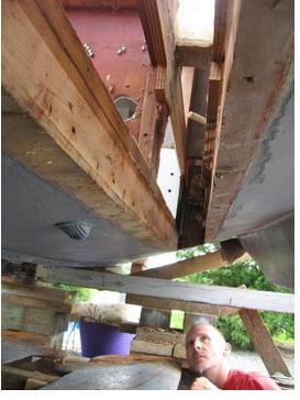
New keel box sides were prepared from 18mm thick plywood, in two pieces, with a scarf joint vertically down each side. Note that once the boat has been built it is not possible to fit a keelbox without removing lots of internal woodwork – including bulkheads – unless you put it in as two pieces as Murray has.
