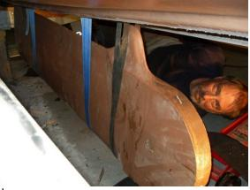
When the keel is high enough I use a jack under the back end and the keel lifting gear to raise it into the slot. When it is in position I check that the holes are lining up by passing a pencil into the keel bolt hole. Don't be tempted to use your finger – if anything slips you will lose it!
