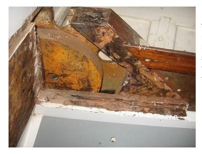
The plywood is cut and chiselled away piece by piece, one side at a time until both sides are totally removed. You can see the blocks which form the front of the keel box in this picture. Ensure that they are in good condition.
