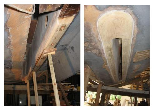
These photos show the new keelbox being assembled , and finished.
