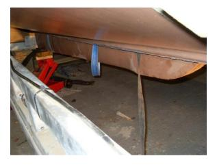
I have a special bush which fits over the end of the main keel bolt to cover the thread, and to act as a taper on the end of the bolt. This aligns the keel as it is pushed (gently hammered) into the hole.
