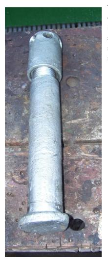
This photo shows a keel bolt and a keel nut. Both are special components. The bolt has a flanged head, with a flat area milled into it. The other end has a Whitworth thread tapped into it, and the special nut fits onto it. The holes in the nut are there to enable a stainless "tommy bar" (slightly bent at each end to clear the support structure) to be inserted and used to turn the nut.
