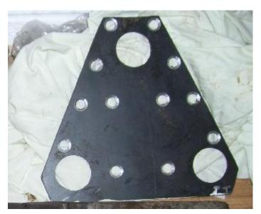
not have this thin plate fitted when new. They had washers under the heads of the bolts.
