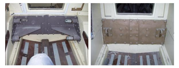
The right hand photo shows it from the aft side of the main bulkhead. This framework passes the stresses from the keels directly through to the main bulkhead, and then distributes it into the structure of the boat.
