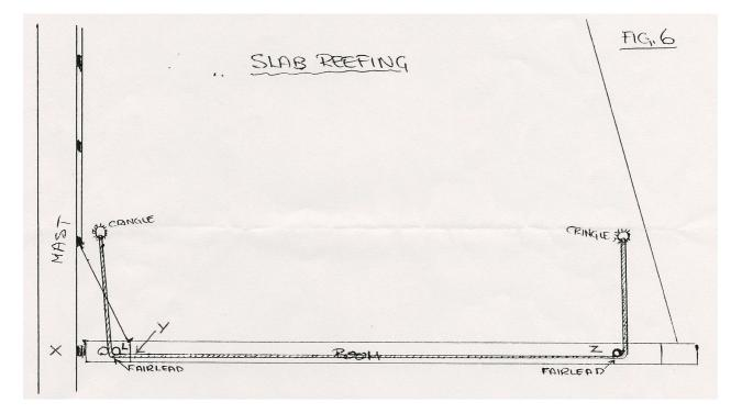
ZIGZAG line show the SLAB REEFING LINE on the Port side where the Main Halyard Gear is on the Starboard side. Thus on the Starboard side and not shown there will be:
