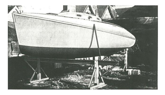
Faced with the problem of removing the Atalanta from its trailer the following apparatus has been constructed. The total cost, including a second-hand hydraulic jack of 4 ton lifting capacity, was approximately £.12. (Rather more these days-Hon Sec)
