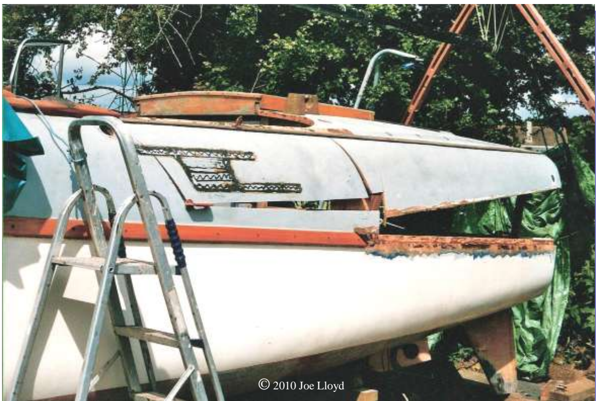
Saw cuts enabled the aft deck to be raised in one piece
