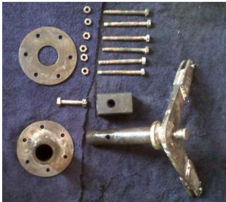
Fig 1b: whipstaff bearing
