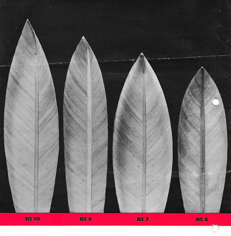
Diagonal "hot-moulding" with approved marine veneer eliminates the old and laborious method of boat-building and permits the advantages of modern construction techniques and production methods to secure the rapid output of almost any hull form.
