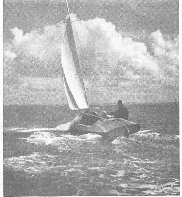
Transom is wider than necessary but gives a stable hull
