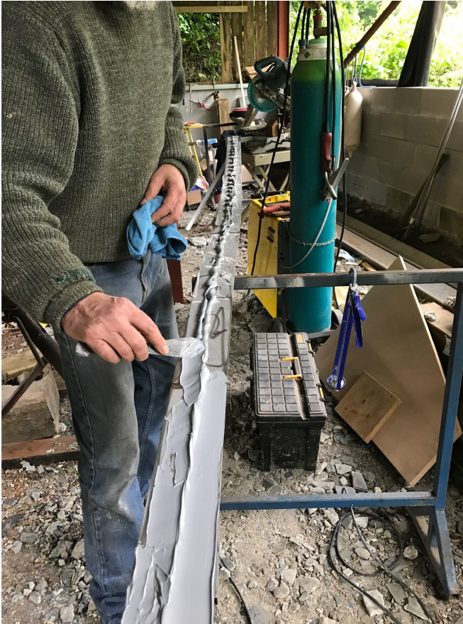
Stainless keel band receiving Sikaflex
