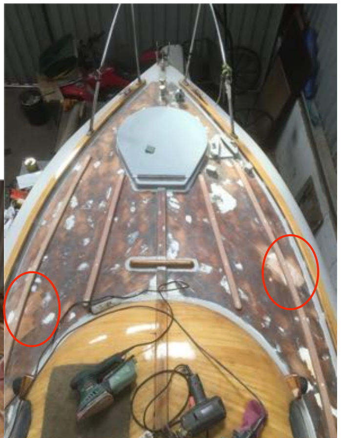
Previous Deck Repairs
