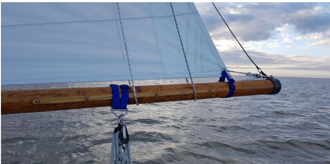
Boom aft, port, showing backing strip for reefing comb and mainsheet attachment
