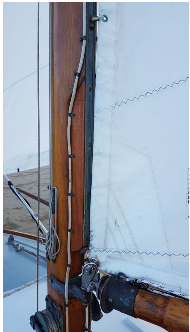
Extension of mast track, closing the gap between slide gate and gooseneck.
