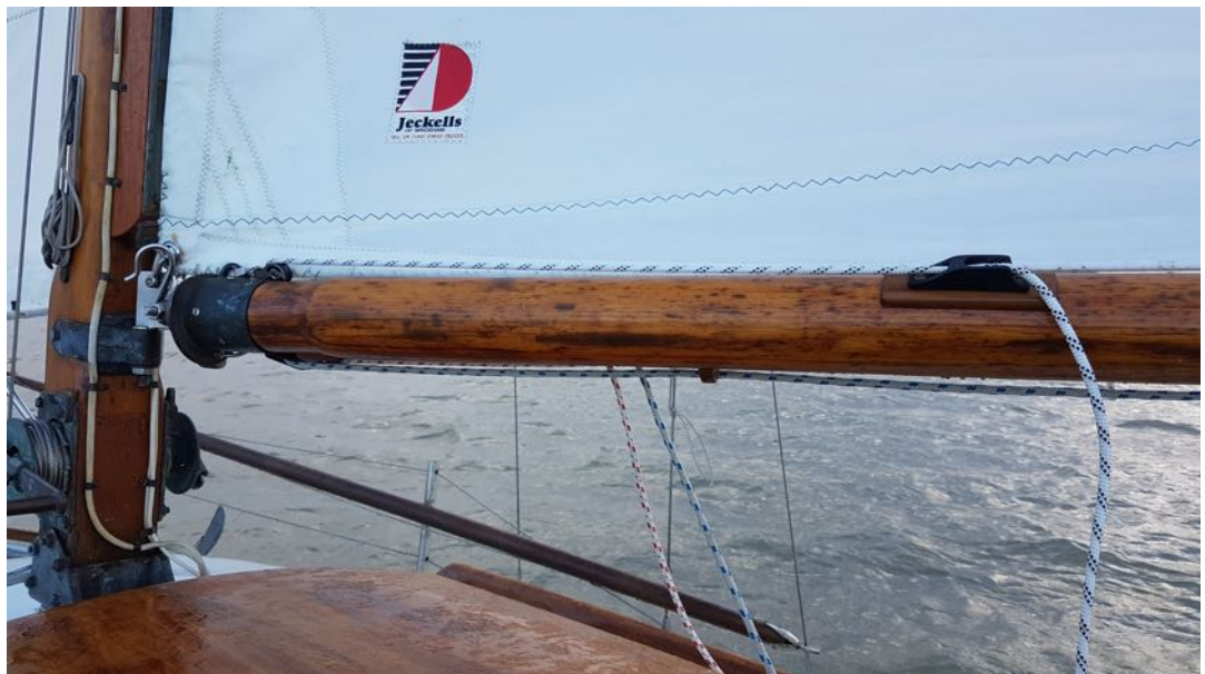
Forward end port showing outhaul cleat, modified roller-fitting and gooseneck
