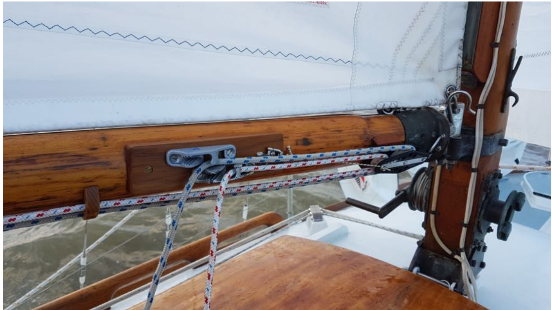
Forward end starboard – reefing line block and cleats, modified roller bronze fitting
