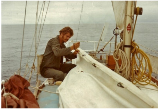
Sail repairs after the storms
