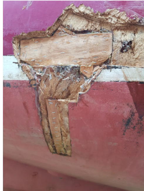
Extensive hull repairs
