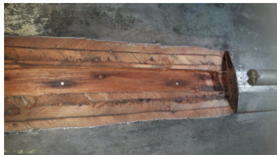
Hull faired off using belt sander
