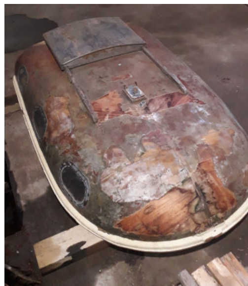
Blister home for repair
