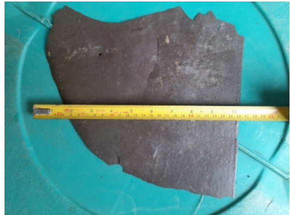
The coating both primer and Coppercoat had flaked off the skeg
