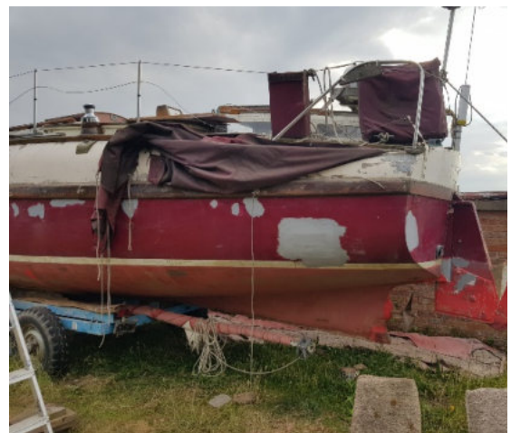
Sanding of filler and top laminate, finally undercoated with primer
