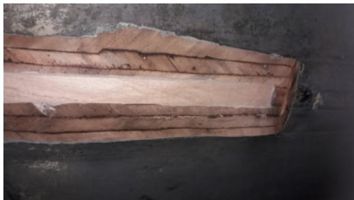
New batten faired off using belt sander
